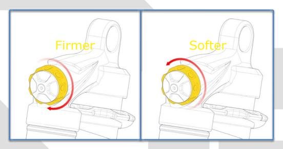
Step 6: High-Speed Compression Adjustment
