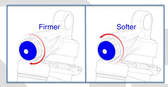
Step 5: Low-Speed Compression Adjustment
