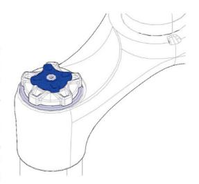
LSC TIP: IF YOU FEEL LIKE THE FORK IS COMPRESSING TOO MUCH DURING BRAKING OR WHEN YOU ARE PEDALING, TURN THE ADJUSTER IN. WHEN ADJUSTING THE LSC, ALWAYS MOVE 2 CLICKS AT A TIME IN EITHER DIRECTION. IF THE CHANGE IS TOO MUCH, THEN BACKTRACK ONE CLICK.
