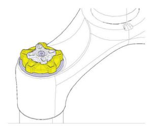
HSC TIP: IF YOU FEEL LIKE THE FORK IS "SPIKING" OR FEELING HARSH DURING FAST, HIGH SPEED IMPACTS TURN THE ADJUSTER OUT A FEW CLICKS. IF YOU FEEL LIKE THE FORK IS GOING TO BOTTOM OUT TOO QUICKLY, TURN THE ADJUSTER IN A FEW CLICKS. WHEN ADJUSTING THE HSC, ALWAYS MOVE 2 CLICKS AT A TIME IN EITHER DIRECTION. IF THE CHANGE IS TOO MUCH, THEN BACKTRACK ONE CLICK.
