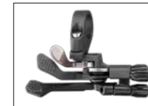
Q Flip 3 Remote Three position 4.7+4.7 Travel WEIGHT: 71g
