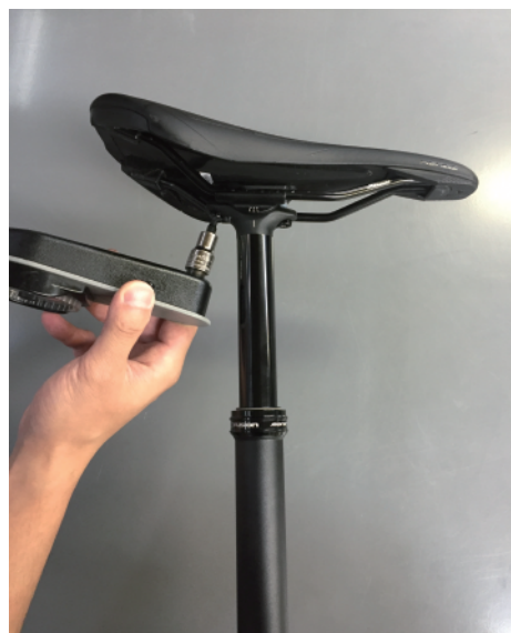
Level Saddle to your preference and Torque bolts to 8 to 10 N-M
