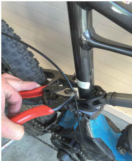
Cut housing at tape mark
