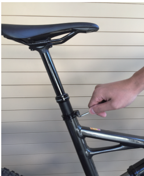
Install to correct height and tighten collar
