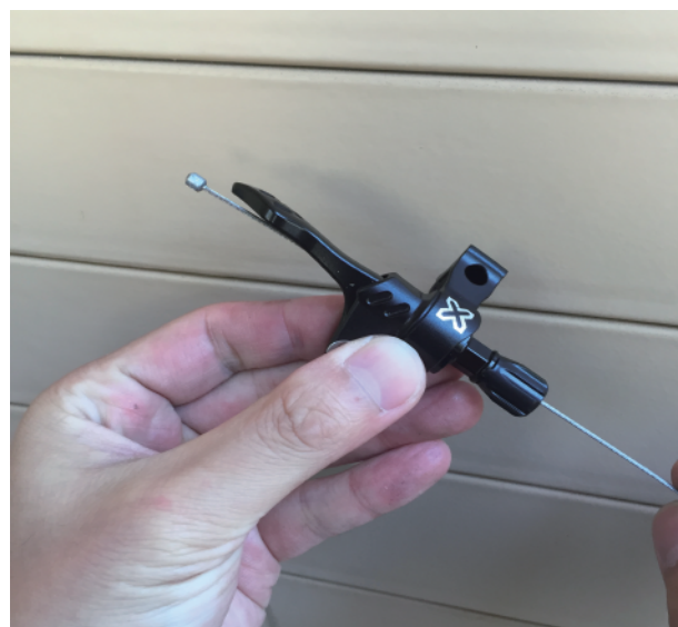
Put cable through remote lever
