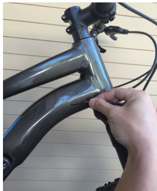
Route housing through frame or attach house per bike manufacturer's specs and install ferrules
