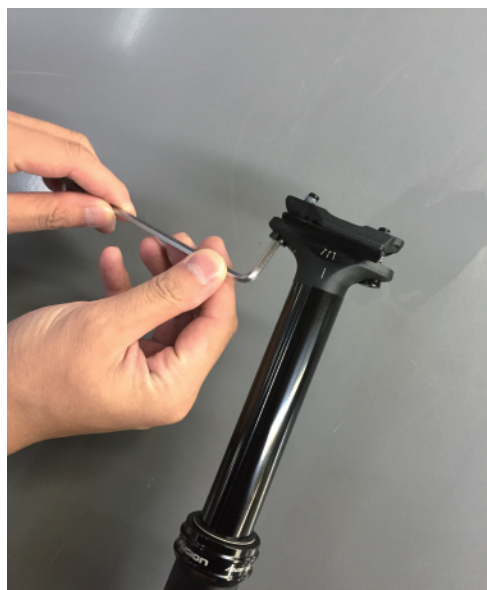
Remove seat post clamp bolts
