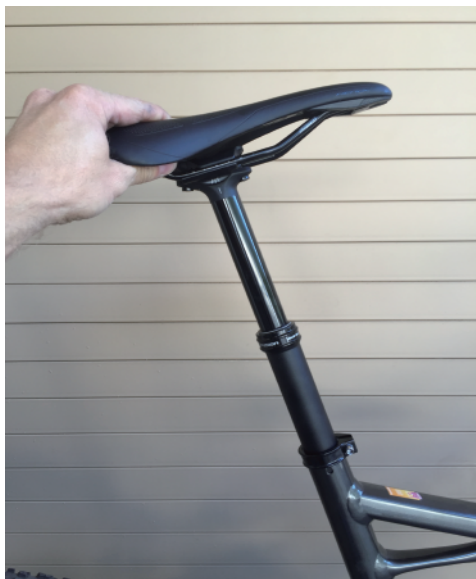
Loosen seatpost collar on frame and install post into frame
