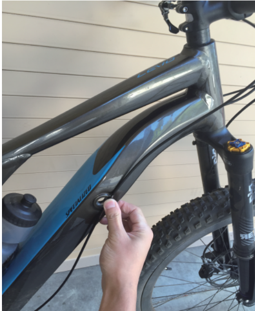
Mimic location the housing would route in frame
